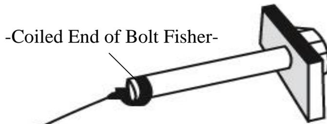
Note: The hardware may vary as to what is being fished along with the bolt. In this instance a 1" X 2" plate washer is being fished along with the hex bolt. Different applications may require fishing through various star washers and flat washers for example.
