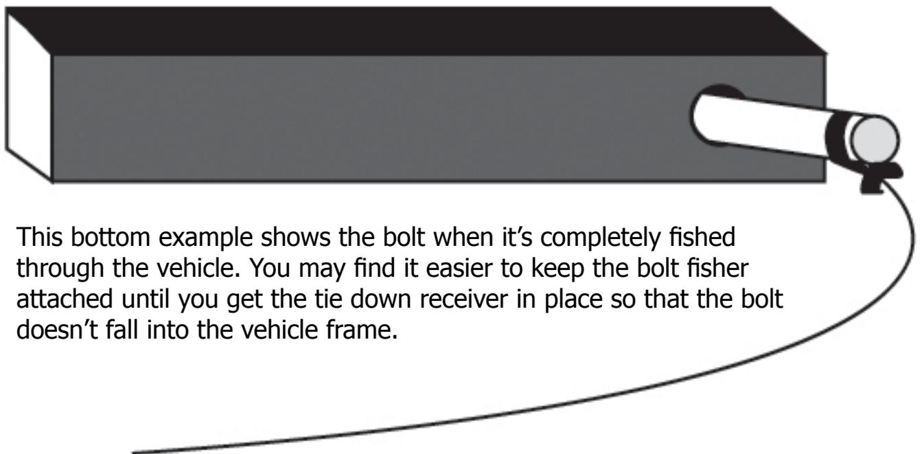
This bottom example shows the bolt when it's completely fished through the vehicle. You may find it easier to keep the bolt fisher attached until you get the tie down receiver in place so that the bolt doesn't fall into the vehicle frame.
