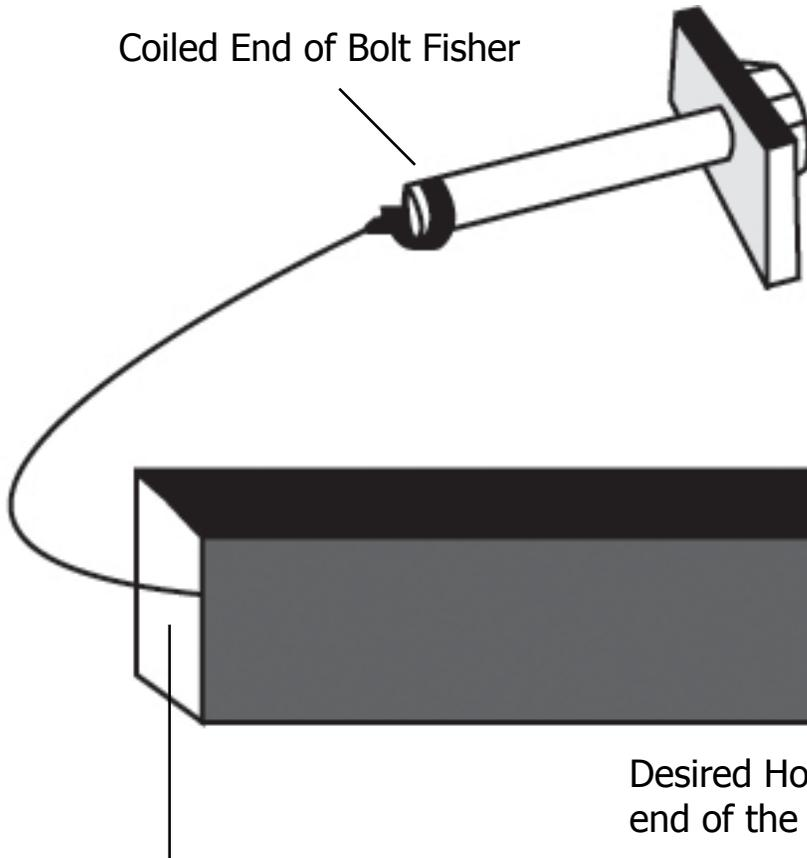
Note: The hardware may vary as to what is being fished along with the bolt. In this instance a 1" X 2" plate washer is being fished along with the hex bolt. Different applications may require fishing through various star washers and flat washers for example.
