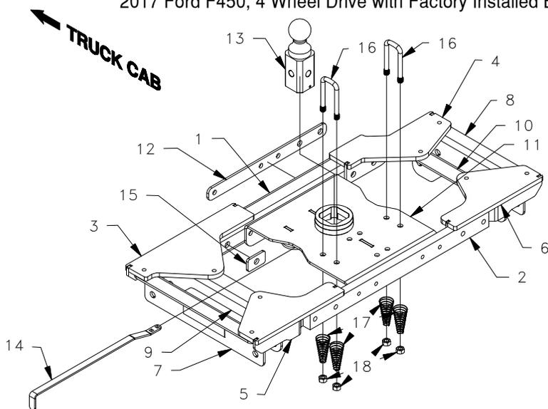
**\*\*NOTE**, Short, 1/2" bolts with thread locker may be flange head bolts with a locking strip, or hex head bolts with red colored thread locker pre-applied.
