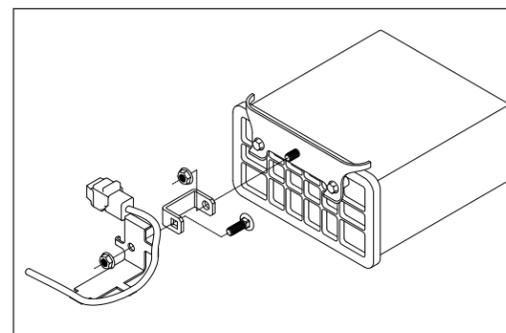
Some trucks may need the exhaust pipe lowered slightly. If the tail pipe has less than 1/4" clearance between it and the hitch use the lowering bracket that is supplied in the kit. Slide it through the lower slot in the rubber hanger and turn downward. This will allow the tube on the tailpipe to slide through the bracket and lower the pipe slightly to give clearance for the hitch. (See diagrams below)
